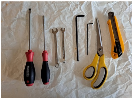
Tools, The most important ones here being 5.5mm socket screw driver (because there are parts on the moulds you just can't reach with normal spanners) 5 and a 2.5mm hex keys and a 10mm spanner.
